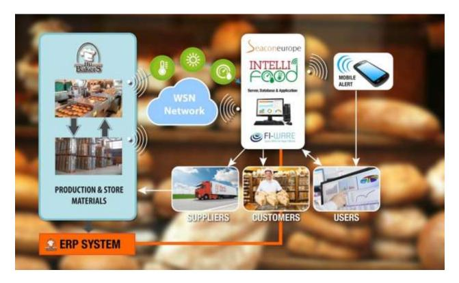
The prepared solution is a system based on wireless sensor network, which is made up of temperature and humidity measurement units (approximately 12-15 sensor points) which are able to communicate with each other. The wiring is not required, the easy to deploy mobile sensors measure the values of the parameters scheduled and communicate the results to a central data store.
